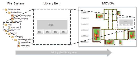
The implemented solution includes the definition of meta-models for library elements and a data structure for managing these elements (see figure above). They contain the presentation, functionality and also the access to the process data server.
